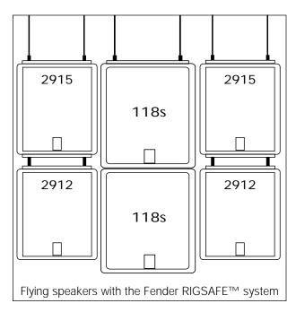
The Fender RigSafe™ system is designed into both speaker cabinets models to safely accommodate such practices. This system is compatible with both the JBL S.A.F.E.™ and the ATM Flyware™ rigging systems. Nonetheless, flying loudspeakers above crowds is dangerous and should only be undertaken by experienced and insured riggers. For more information on safe rigging practices, please refer to the "Flying with Fender RigSafe™" brochure (p/n 049646) or contact ATM FlyWare at (310) 834-5914.
